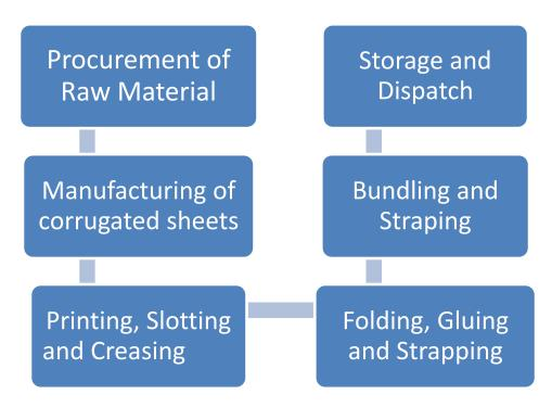
Our manufacturing process starts with procurement of raw materials i.e. Kraft Paper, adhesive for Ply bonding, adhesive for glue tab and water based ink. Kraft Paper is arranged from paper mills in the form of reels as per the requirement of customer based on the GSM requirement of carton. Adhesive for ply bonding is manufactured in our manufacturing facility which uses a controlled input of native
