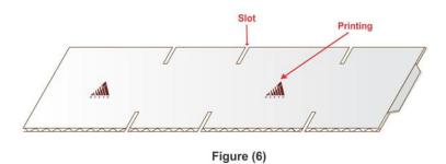
Printed and slotted sheets from the printing machine are then passed on to the feeding section of standalone folder gluers which then apply glue on the glue tabs and fold sheets to form a box (as specified in figure 7 and 8). These boxes are then bundled and strapped together by the auto ejector and strapping machine (as specified in figure 9). These bundles are then stacked one above the other upto a optimal height and are now ready to dispatch.
